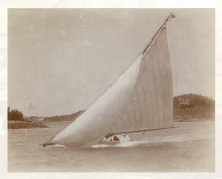
A small Bermuda sloop with the classic "Bermuda Rig" (fore and aft sails) used by most modern yachts and invented in Bermuda before 1674 (Photo takenabout1910).
